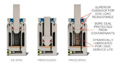
The patented dynamic lubrication system coats the gas spring wall, piston and seal with oil on every stroke of the press to reduce heat build-up and lower operating temperature, which in turn, reduces wear on die components and extends performance life.
